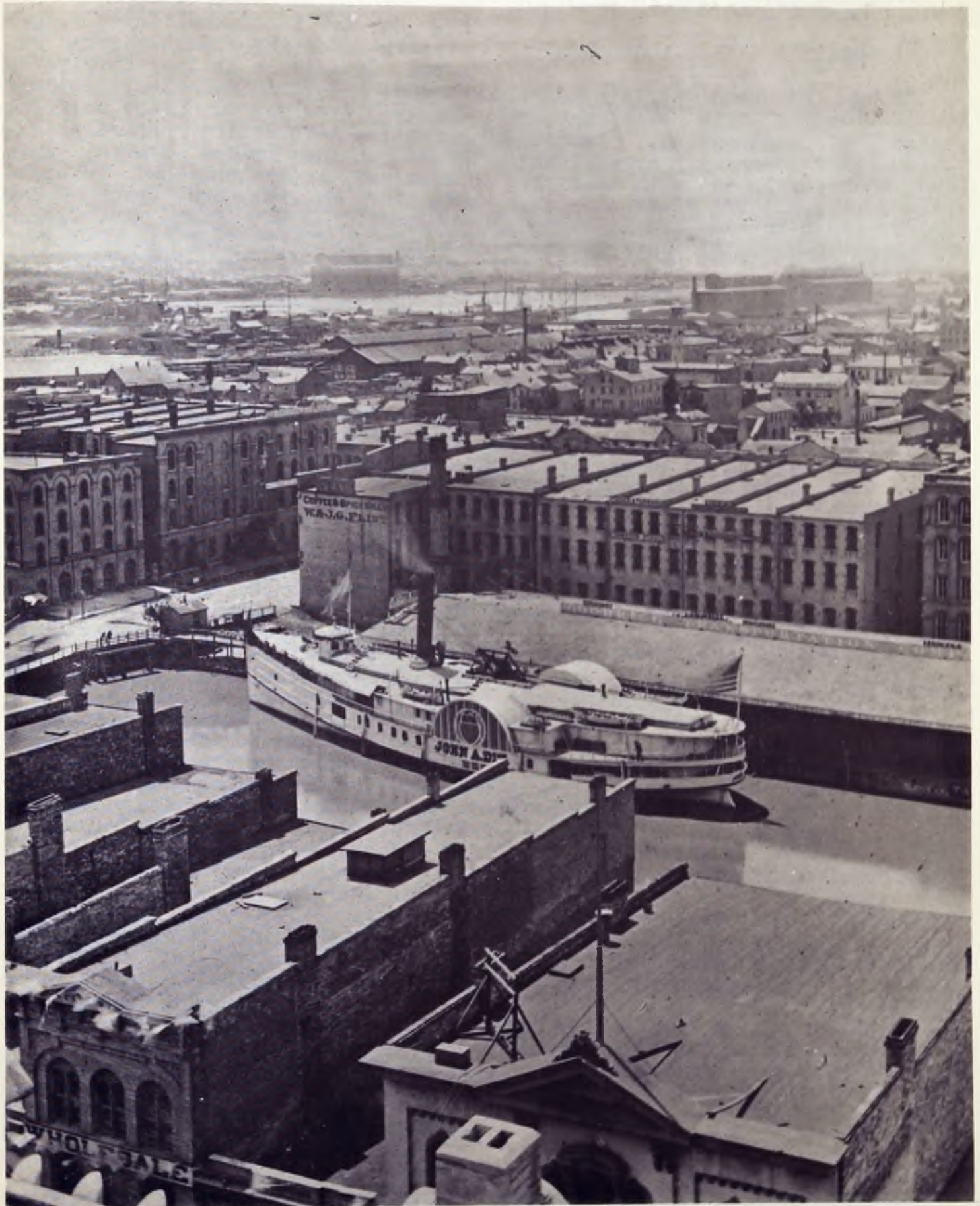
Steamer John A. Dix, owned by Eber B. Ward Built 1865. 172 Ft. long. 527 Gross tons.
