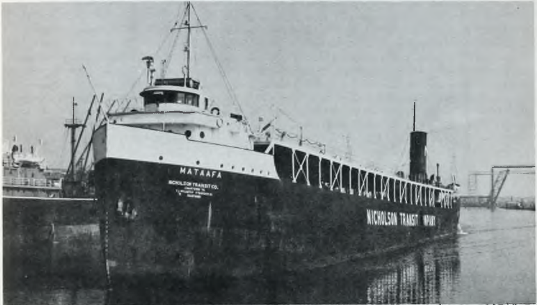
MATAAFA(b), Pennsylvania(a) US# 150810 Gr. T. 4775 N.T. 3957, 437'8 \frac{1}{2} "x50x28'7 \frac{1}{2} " Built by Cleveland S.B. Co. hull # 33 at Lorain, Ohio in 1899. Quad. Exp. Eng. 16-23 \frac{1}{2} -36 \frac{1}{2} -56x40 blt. by Cleve. S.B. Co. in 1899. 2 water tube boilers blt. 1927. Owners (1) Minn. S.S. Co. (2) Pittsburgh S.S. Co. (3) Ecorse Transit Co. (4) Nicholson Transit Co.
