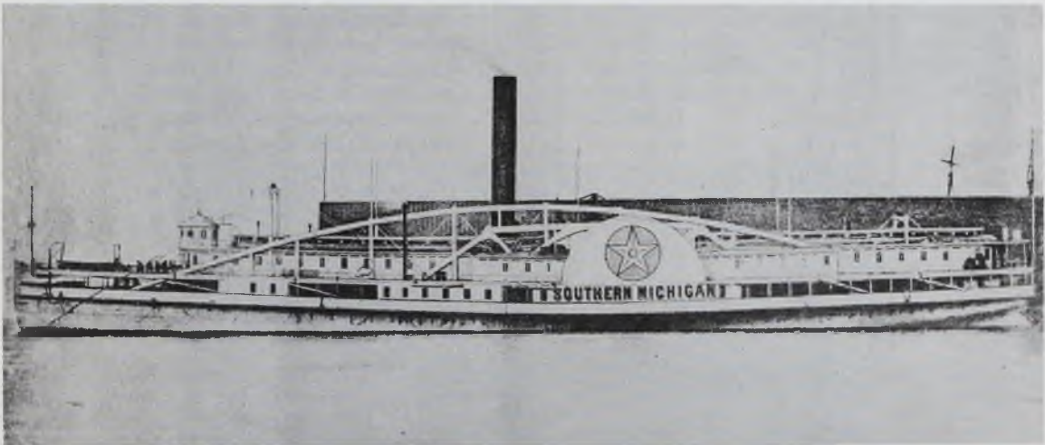
Passenger Sidewheel SOUTHERN MICHIGAN. Built at Buffalo, New York in 1852 by Bidwell & Banta. 300.9 x 36.11 x 13.7. Tonnage (old) 1470, built of wood. Her engines were vertical beam, 72 diameter, by 144 stroke, built by Morgan Iron Works, in 1852. She was owned by Michigan Southern Ry. Dismantled in 1863.
