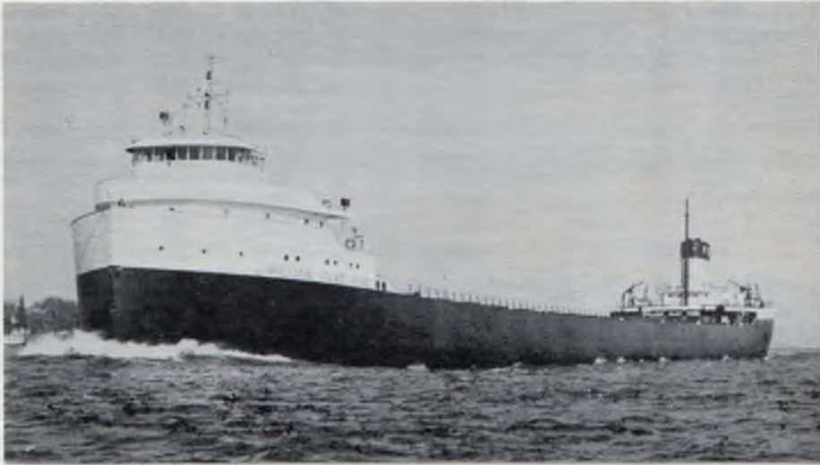
WILLIAM CLAY FORD US# 266029 GT. 11590 NT. 8590 629x70x36 Built by Great Lakes Eng. Works, hull #300 at River Rouge, Michigan. Launched Aug. 1953. She has a Westinghouse Electric Co. 2 cyl. stm. turb. of 7700 SHP and Foster-Wheeler boilers. Owned by the Ford Motor Co. of Dearborn, Michigan
