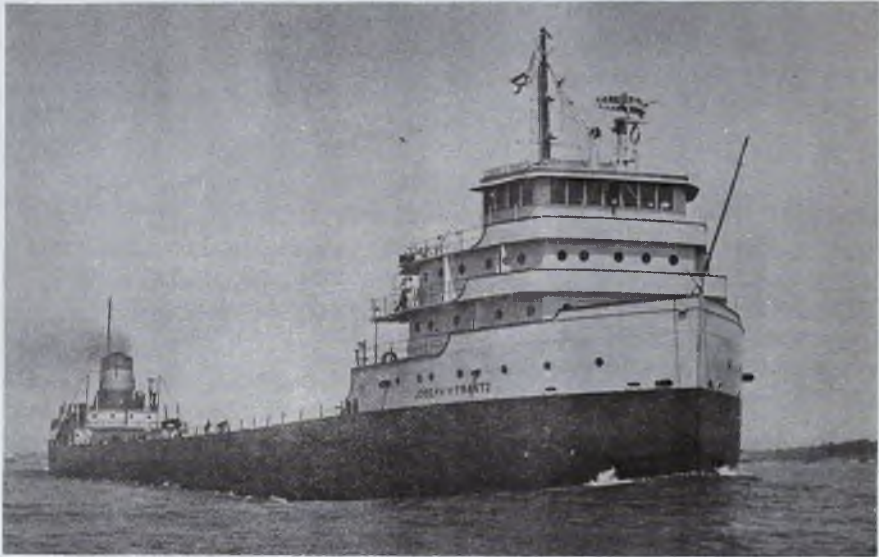
JOSEPH H. FRANZ. US 224409. G.T. 8289, N.T. 6436. 600'11" x 62' x 32'. Built by Great Lakes Engineering Works in 1925, hull no 248. Originally had triple expansion engine but was re-powered in 1955 with a 5325 I.H.P. Skinner Engine and 2 new B & W water tube boilers. Owner: Columbia Transportation Company.
