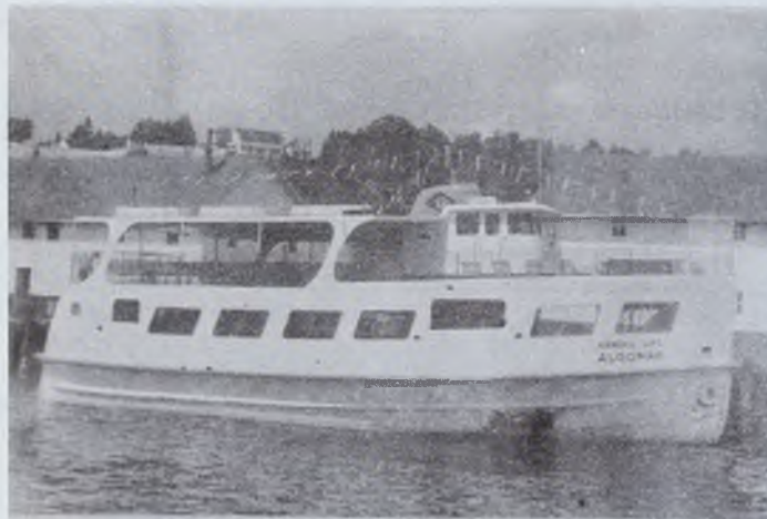
ALGOMAH. 65'x 30'x 7' (MV). Built 1961, for Arnold Transit's service, between Mackinac City and Island. She is duplicate of OTTAWA, built in 1959 and is rated 400 passengers.
