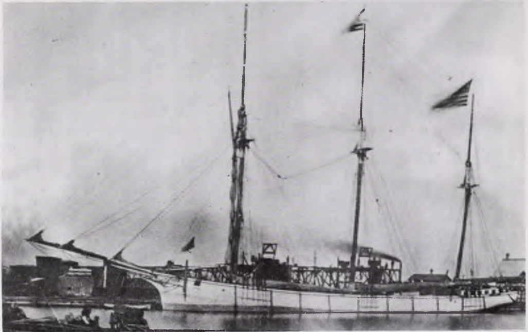
Top: J. I. CASE (US 75720, later Can. 141595). 1874 Manitowoc by Rand and Burger for J. I. Case Plow Works Co., Racine, Wis. 208 x 34 x 15. J. I. CASE had the tallest spars of any vessel upon the Great Lakes. Her mainmast stood about 190 feet above water line.
