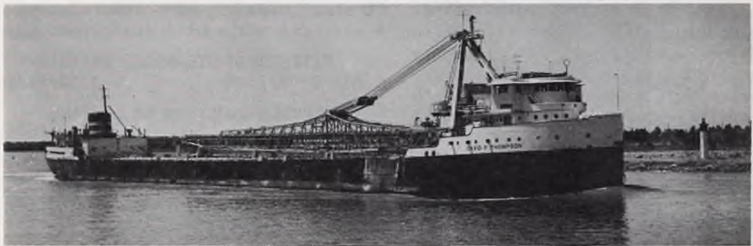
Among repowered older lakers, David P. Thompson (above) has a Skinner-Unaflo engine, with cabins aft much rebuilt in her conversion. William G. Mather (below) was given geared turbines and now has fully-automated boiler controls.
