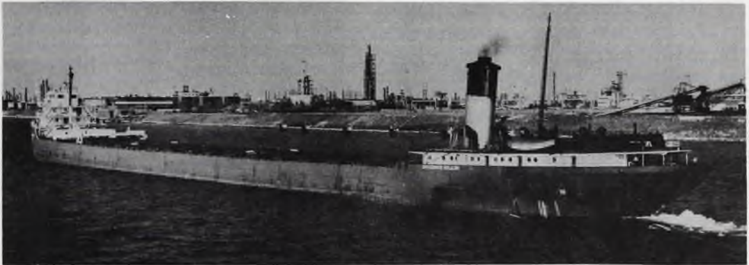
Carl D. Bradley of 1927 (above) had a turbo-electric drive, while Governor Miller (below) was one of four near-sisters of 1938 to introduce geared turbine propulsion to lakers.
