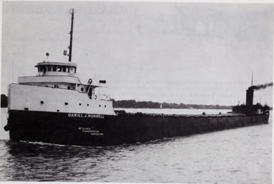
In Bethlehem colors in the late Forties, the MORRELL is seen downbound on the Detroit River. Her new pilot house and texas, added in the thirties, is seen here.
