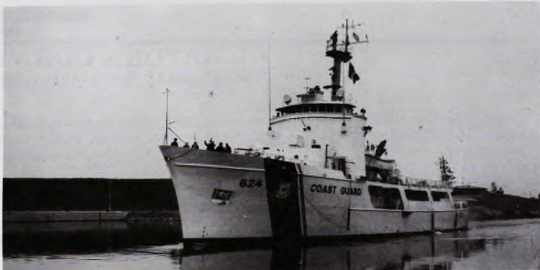
U.S.C.G. DAUNTLESS at Iroquois, downbound June 16, 1968. She is Diesel twin-screw medium endurance cutter #624, built by American Ship (hull 884). Dimensions: 210' x 34' x 19½'.
