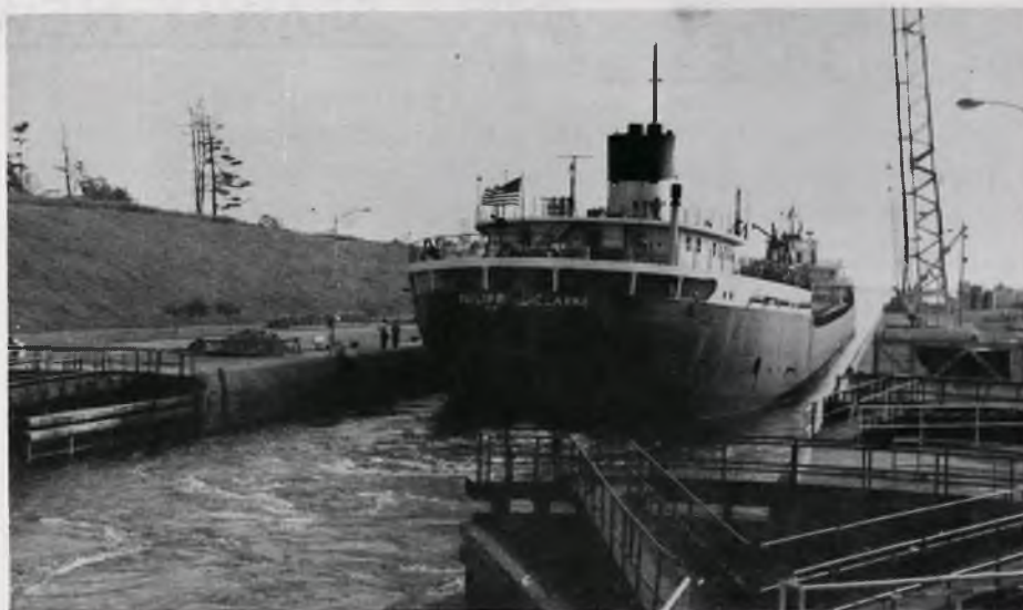
PHILIP R. CLARKE makes an unusual non-stop run through the Iroquois Lock. Water levels permitted both gates to be open at the same time. Photo by GEORGE AYOUB
