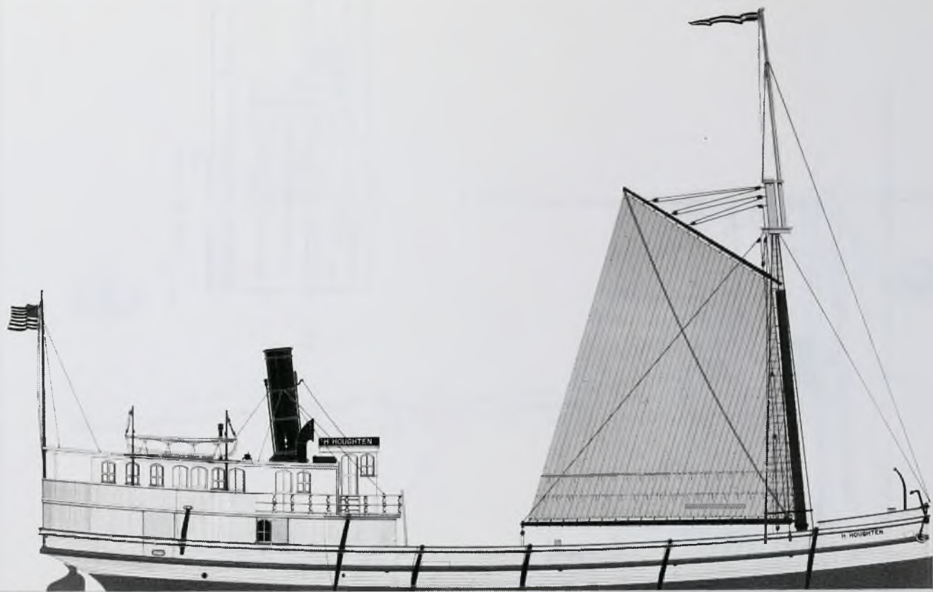
H. HOUGHTEN - U.S. 96006 LENGTH 120' BEAM 27' DEPTH 8.5' BUILT 1883 BY F.W. WHEELER & CO. AT WEST BAY CITY, MICHIGAN FOR H. HOUGHTEN OF DETROIT, MICHIGAN. THE ENGINE BEING OF THE FINE 8 HPT COMPOUND TYPE WAS BUILT BY J.E. WILSON OF DETROIT. SHE SPENT MANY OF HER YEARS CARRYING LIMESTONE AND GENERAL CARGO UP AND DOWN THE ST. LAIR AND DETROIT RIVERS ON NOVEMBER 20, 1928 THE H. HOUGHTEN BURNED IN THE RIVE BONA CHANNEL, ST. LAIR RIVER.
