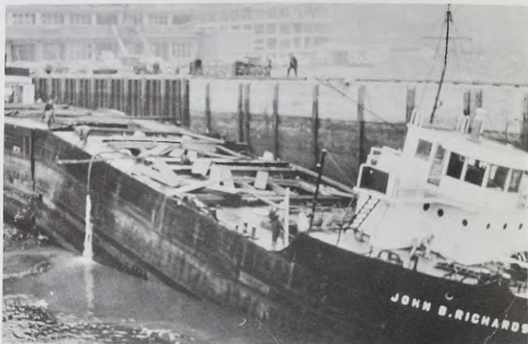
JOHN B. RICHARDS with hull broken at St. John, New Brunswick.
