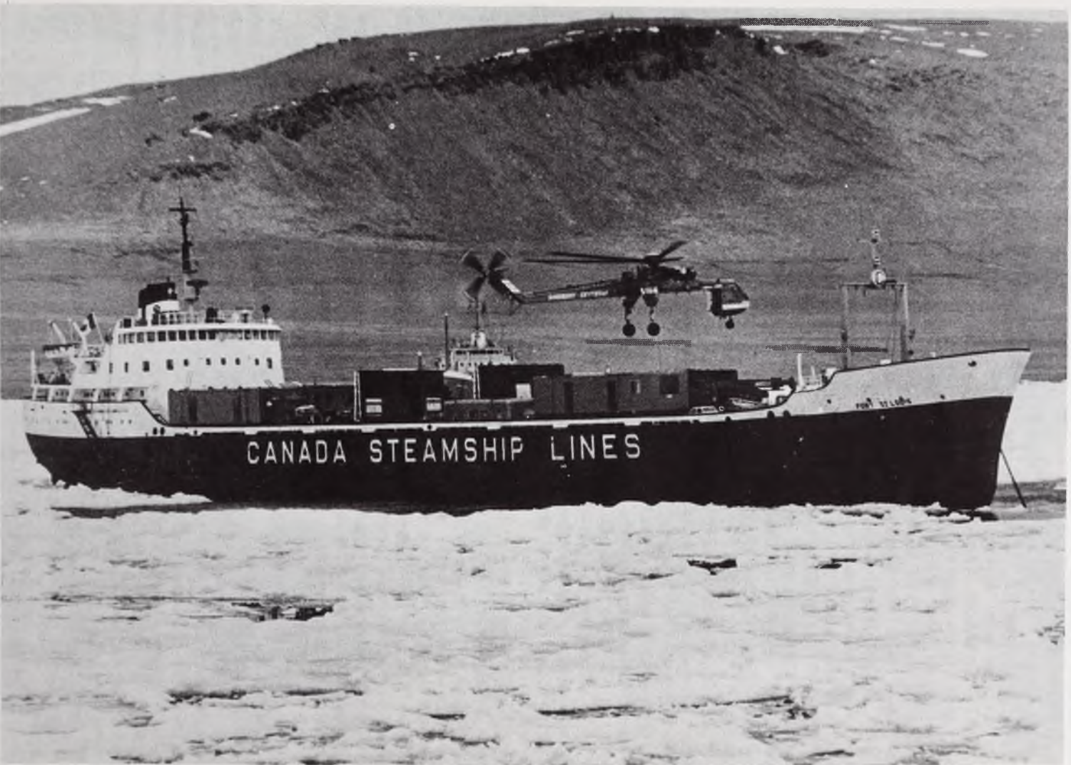
Skycrane extracts cargo from hatch of FORT ST. LOUIS , anchored off Resolute. Ice would have banned normal lightering methods.
