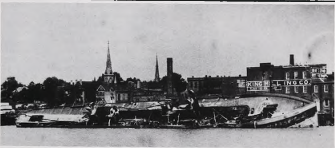
Flooded by streams of water from fire hoses, the UNITED STATES settled to the bottom and heeled over on her starboard side, a burned out hulk. Author's Collection.
