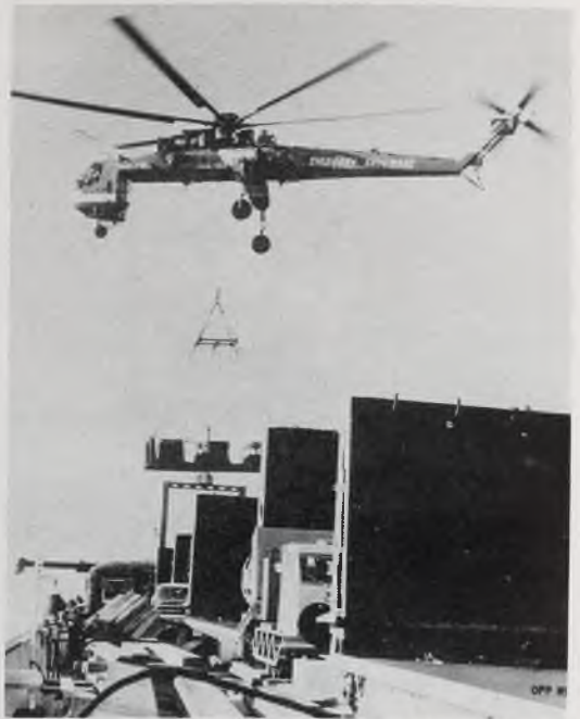
At Pond Inlet, Skycrane hovers 65 feet above hatch to lift gondola for delivery to village ashore. Drop zone was about a mile from the ship.
