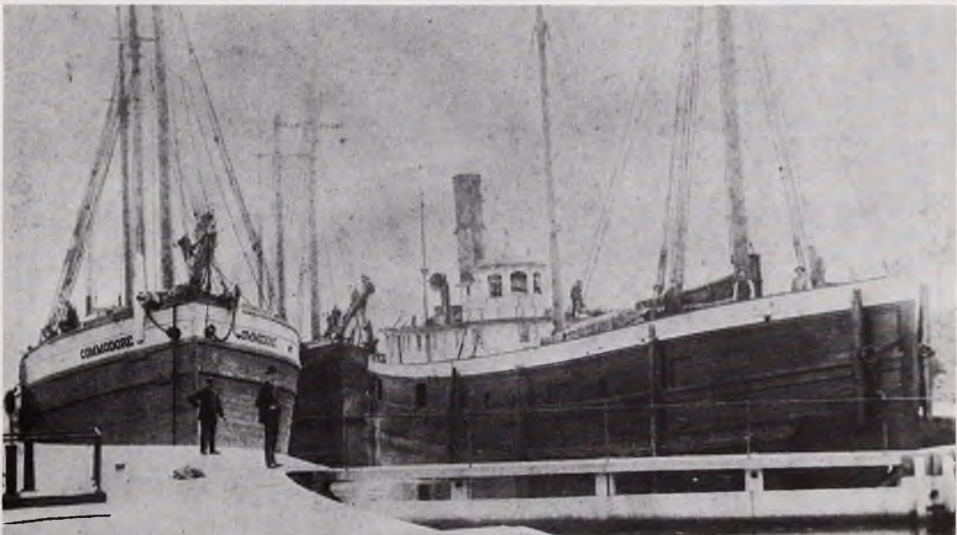
Although built in the "rabbit" profile, P. H. BIRCKHEAD of 1870 was originally a decked ship with side ports as shown in an early view. The schooner COMMODORE is beside her in the canal lock, with the schooner C. B. JONES beyond.
