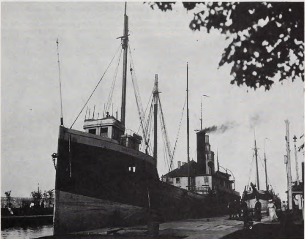
This later view of P. H. BIRCKHEAD shows the vessel converted to a bulk-freighter with a pilot house now on a raised forecastle. Beyond is her tow, the schooner-barge CHARLES A. BURTON.
