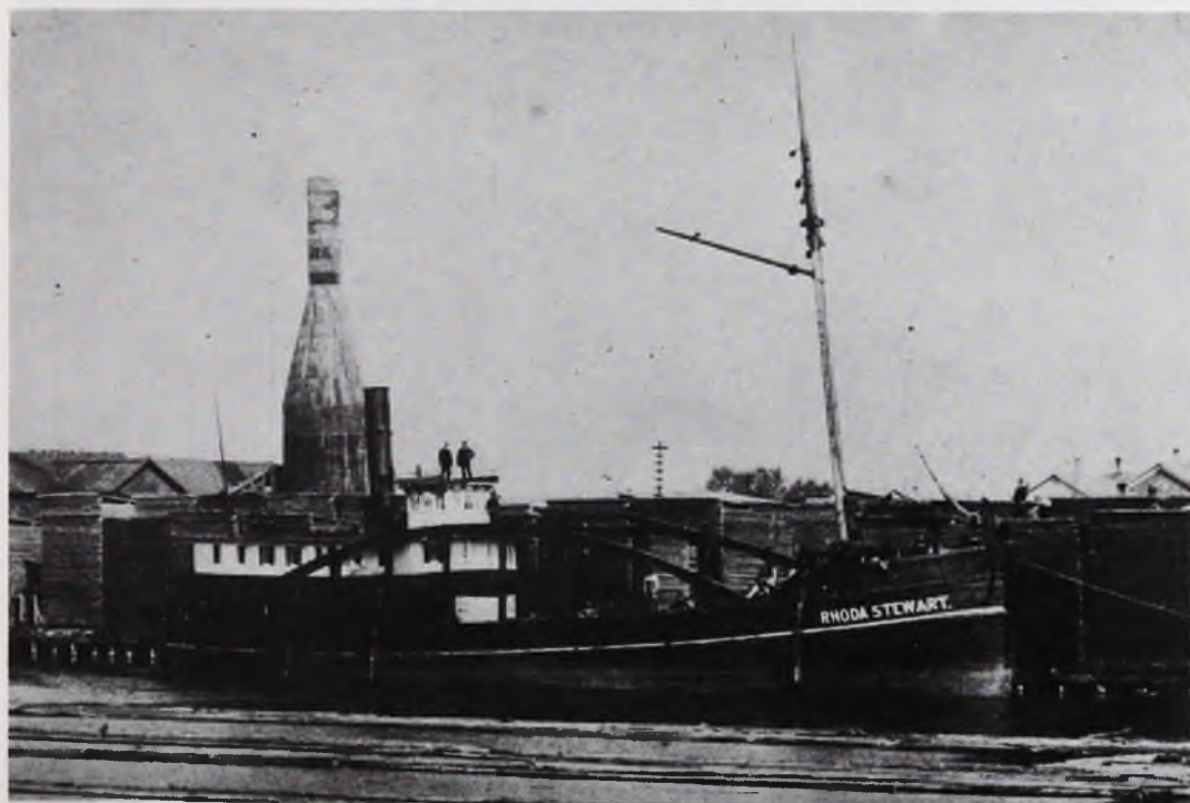
Even after larger bulk freighters of the new fashion had appeared, rabbits continued to be built for the lumber trade. RHODA STEWART was built at Algonac with high hogging arches obstructing her cargo deck.
