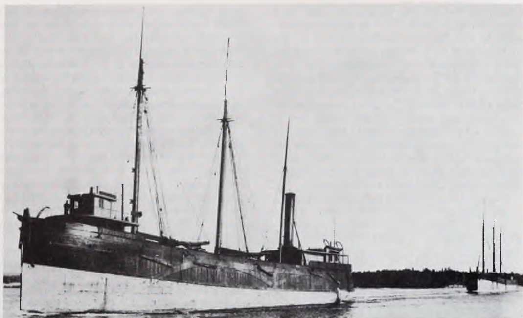
Originally a barge consort to R. J. HACKETT, the FOREST CITY soon became a steamer closely resembling the HACKETT. In this view with the WILLIAM MCGREGOR in tow, FOREST CITY retains much of her original rigging, and the arch-like stiffening of her hull is quite apparent.
