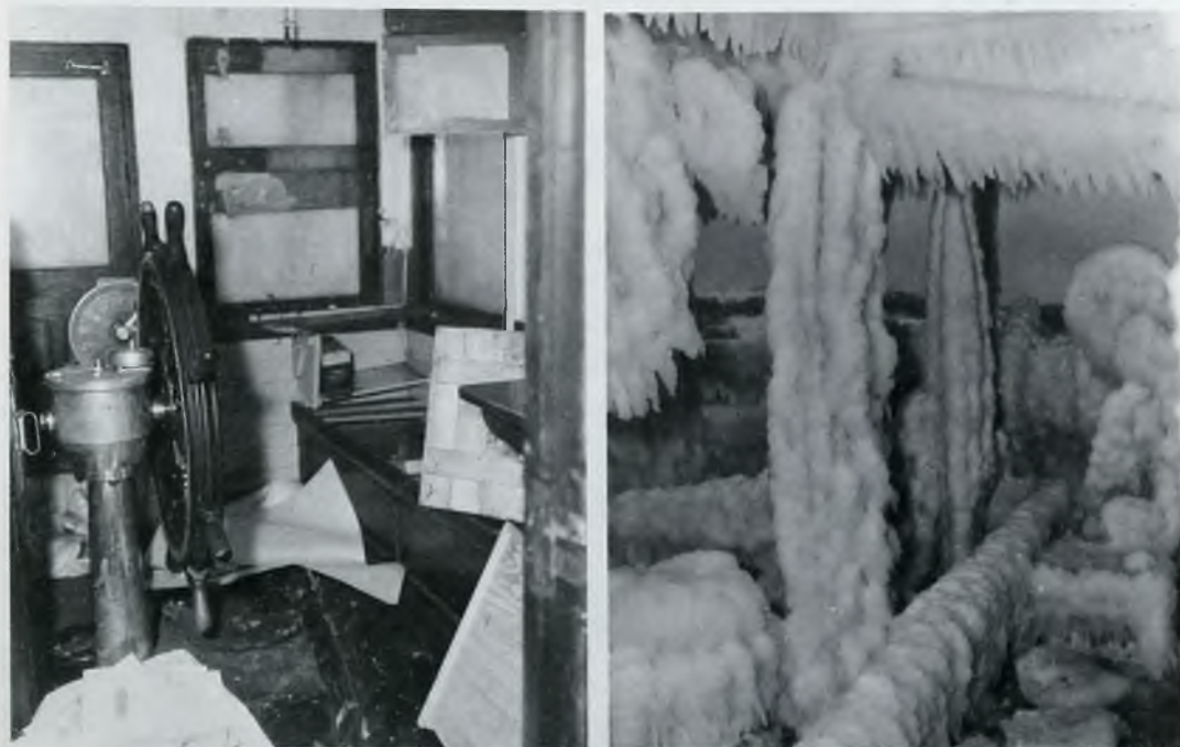
The wheelhouse (left) seen through port doorway, and intolerable weather conditions are evident in the ice on winch, winch cage and mooring line (right).
