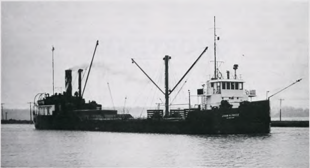
A revitalized JOHN H. PRICE at Lock 19, Cornwall Canal, 29 April 1956. Note the new wheelhouse.
