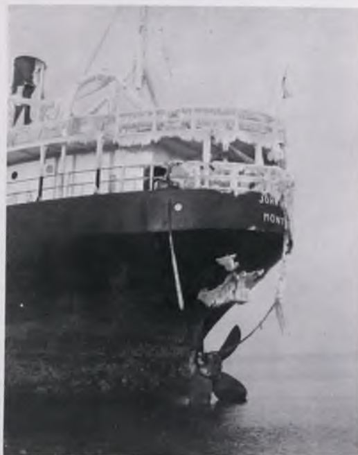
Stern, showing rudder missing and lines fouling propeller.
