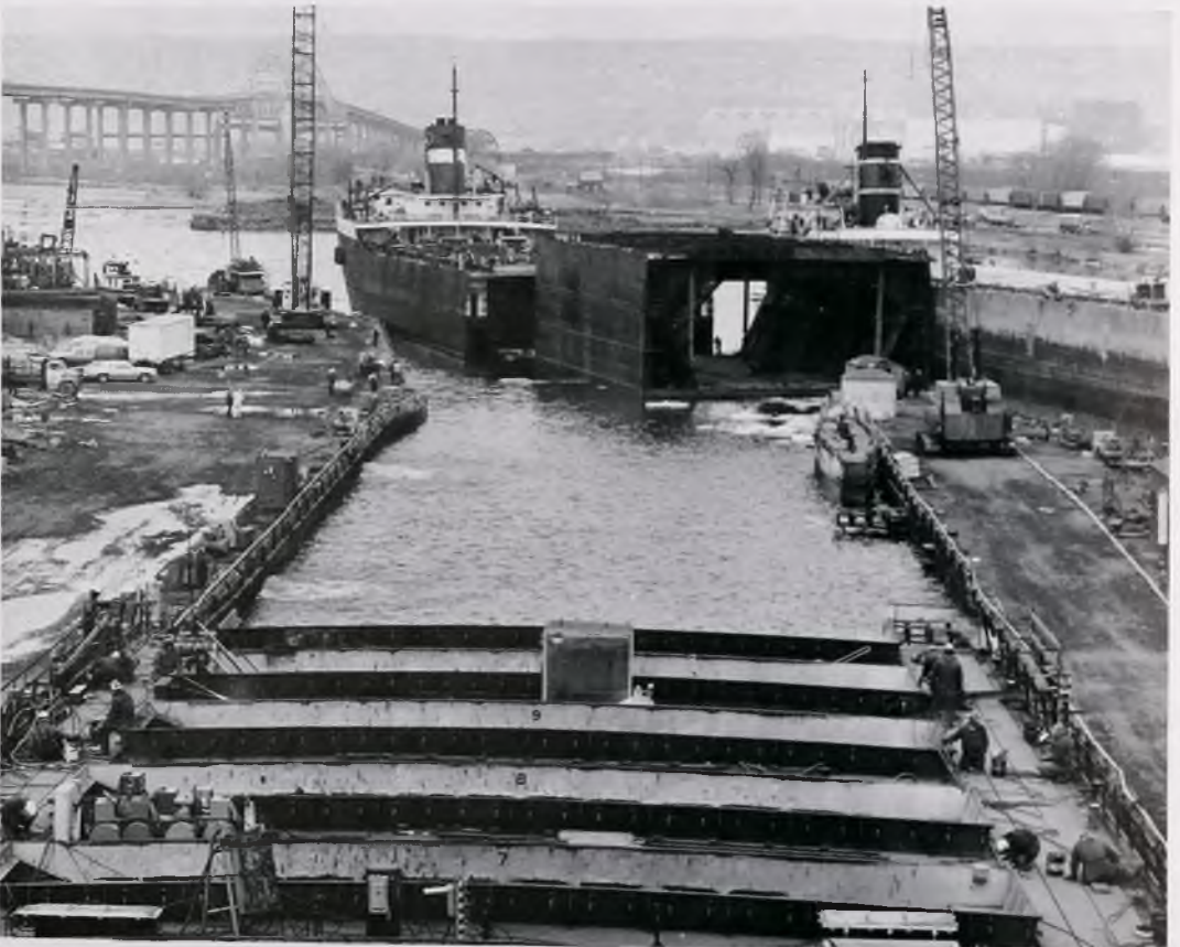
Like a giant jigsaw puzzle, the three pieces of WILLIAM CLAY FORD were fitted together in an elaborate lengthening process at Fraser Shipyards, Superior, Wisconsin. Floating higher than the bow (foreground) and stern, which were ballasted and watertightened in drydock, is the new 120-foot steel mid-section. A crew of 120 tradesmen — including boilermakers, carpenters, welders, machinists, electricians and crane operators — working three shifts several days in April [1979] welded the ship together and installed a new stern thruster to improve maneuverability. The first Ford vessel to be lengthened, the ship was cut in half, the dock flooded, and the new midsection floated in. The three "pieces" were then welded together, water tested, and painted.
