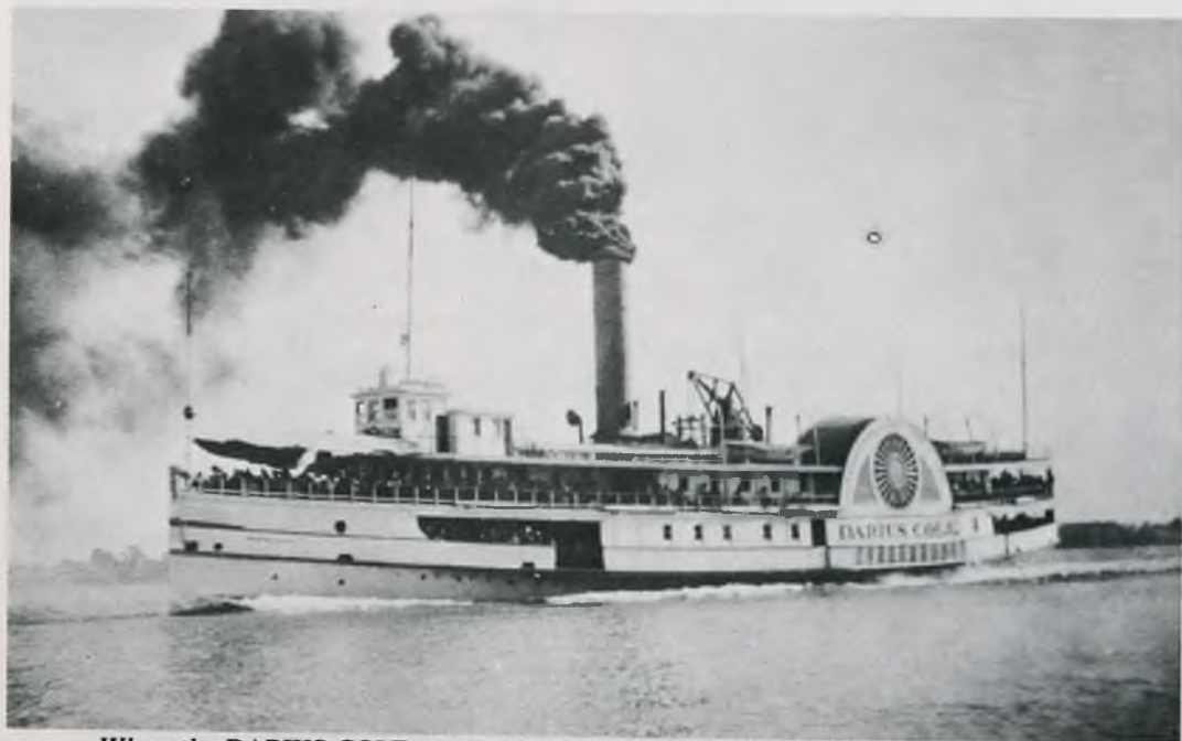
When the DARIUS COLE was built, she was considered a "safe ship" because her boiler and engine room were enclosed with heavy iron.
