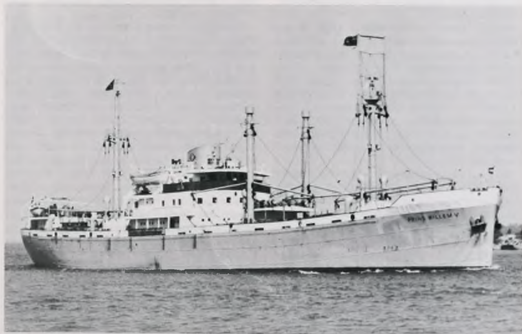
The PRINS WILLEM V was built for the lake trade and was lengthened when the Seaway was opened.
