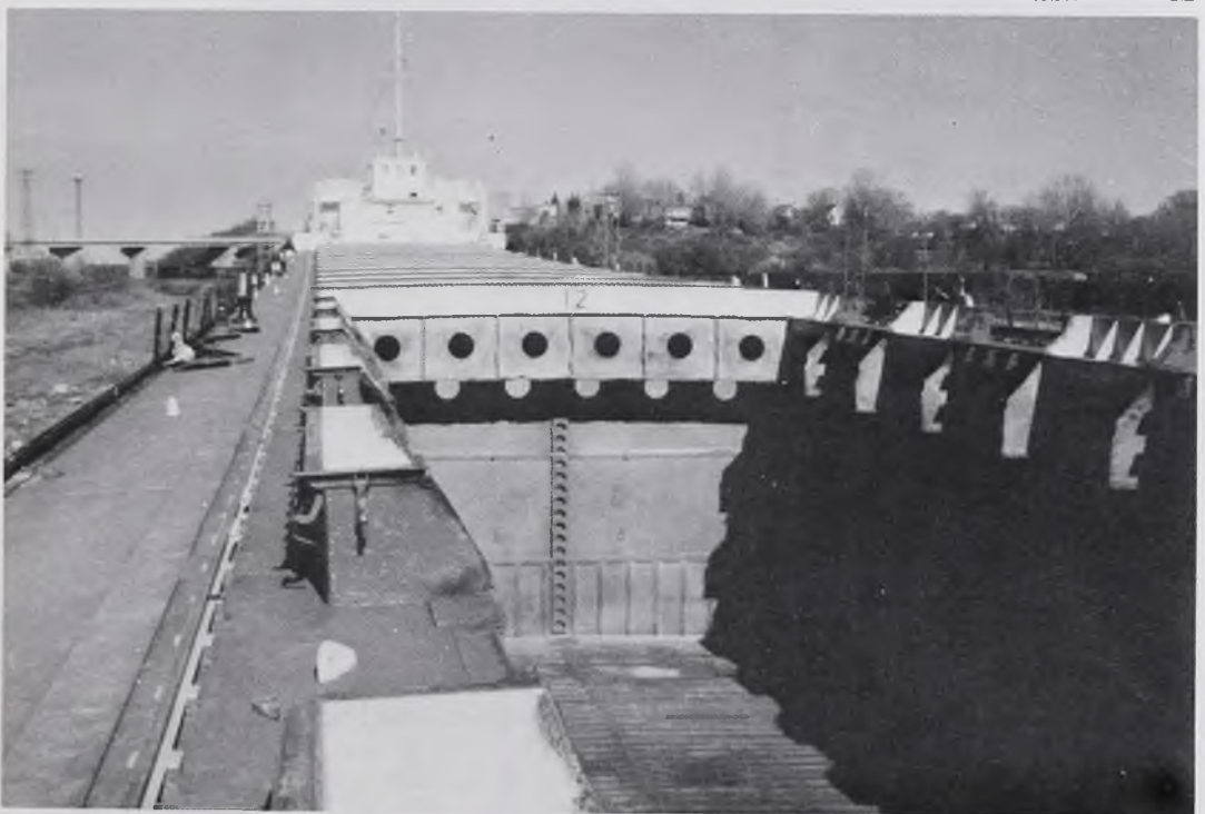
The hatch covers were the first to go as the scrapping of the HEIMBECKER begins.
