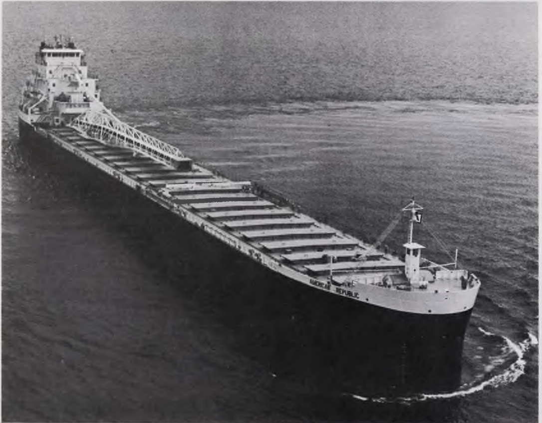
The AMERICAN REPUBLIC, 634 x 68 x 40, is powered by twin screws so the engine room could overlap the cargo hold and save space.
