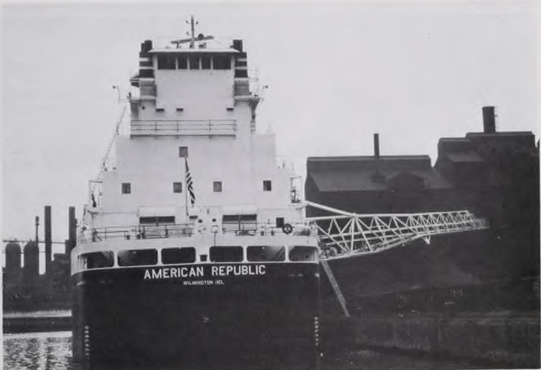
The pilot house has a step formation at the forward rather than after part to give the captain the best view over the stern while backing.
