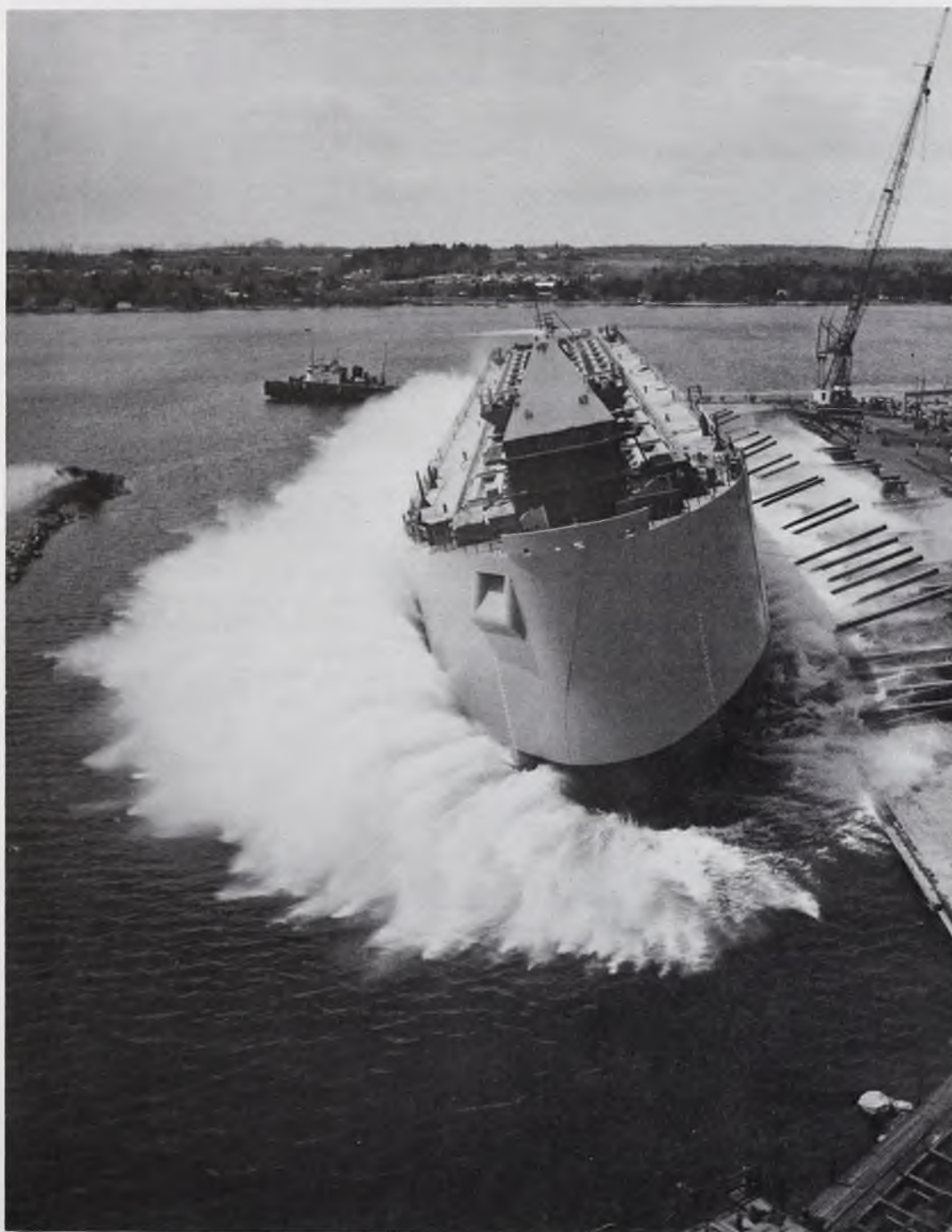
Launching of HULL 728, the largest known self-unloading phosphate barge in the world. Measuring 610-feet, the ocean service barge will have a capacity of 42,000 DWT tons. The barge is being built for Beker Shipping Company of Greenwich, Connecticut.
