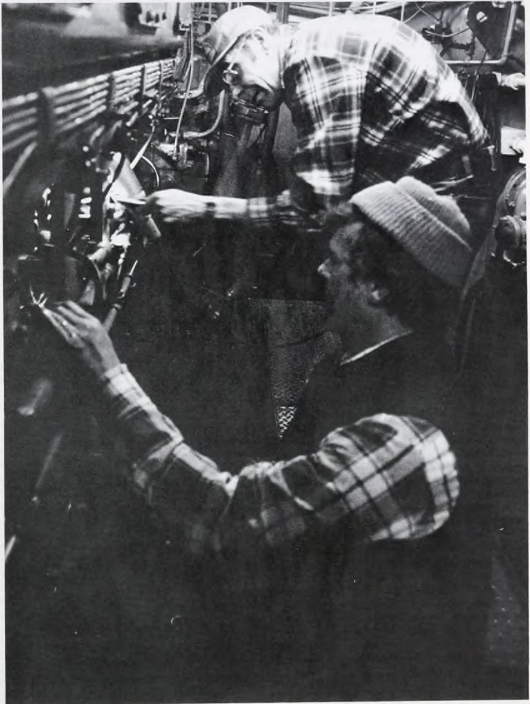
Engineer Walter White and assistant engineer Charlie Newell make a quick running repair on the 2000 hp Fairfax engine.
