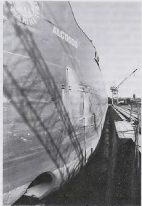
In drydock, the bow thruster is clearly visible.
