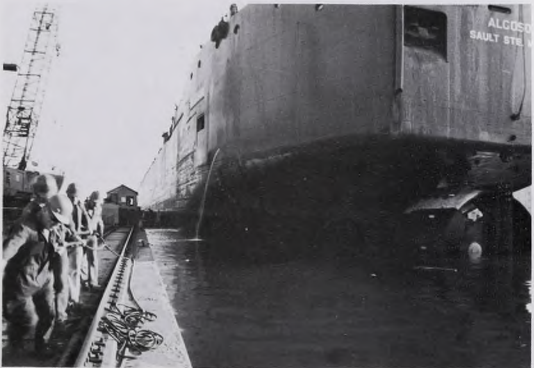
The ALGOSO being winched into the dock after the tugs no longer have room to maneuver her.
