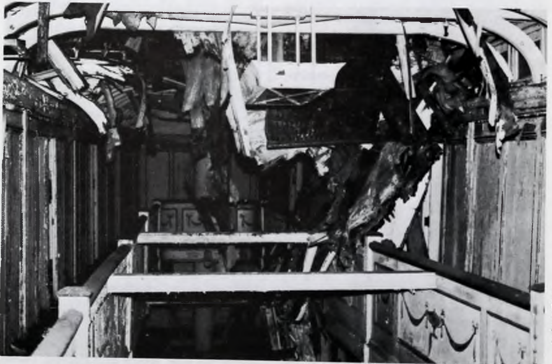
The cabins of "A" deck have fallen through to the gallery below on "B" deck.
