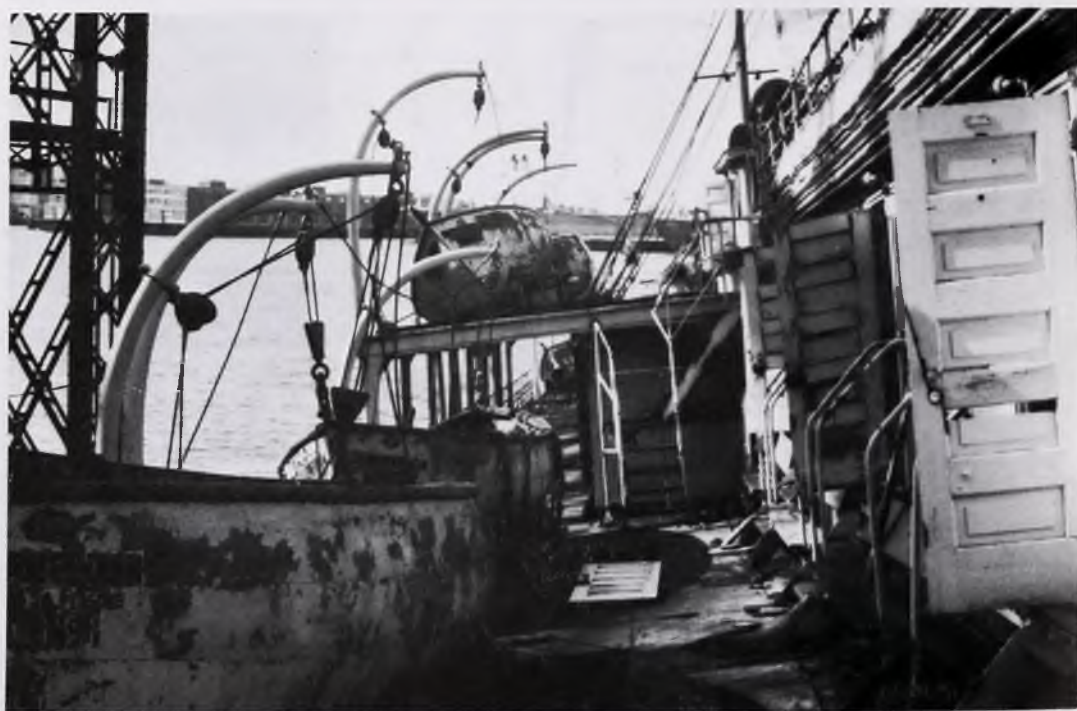
The lifeboats rest at various angles, slowly forcing their weight down through the deck.
