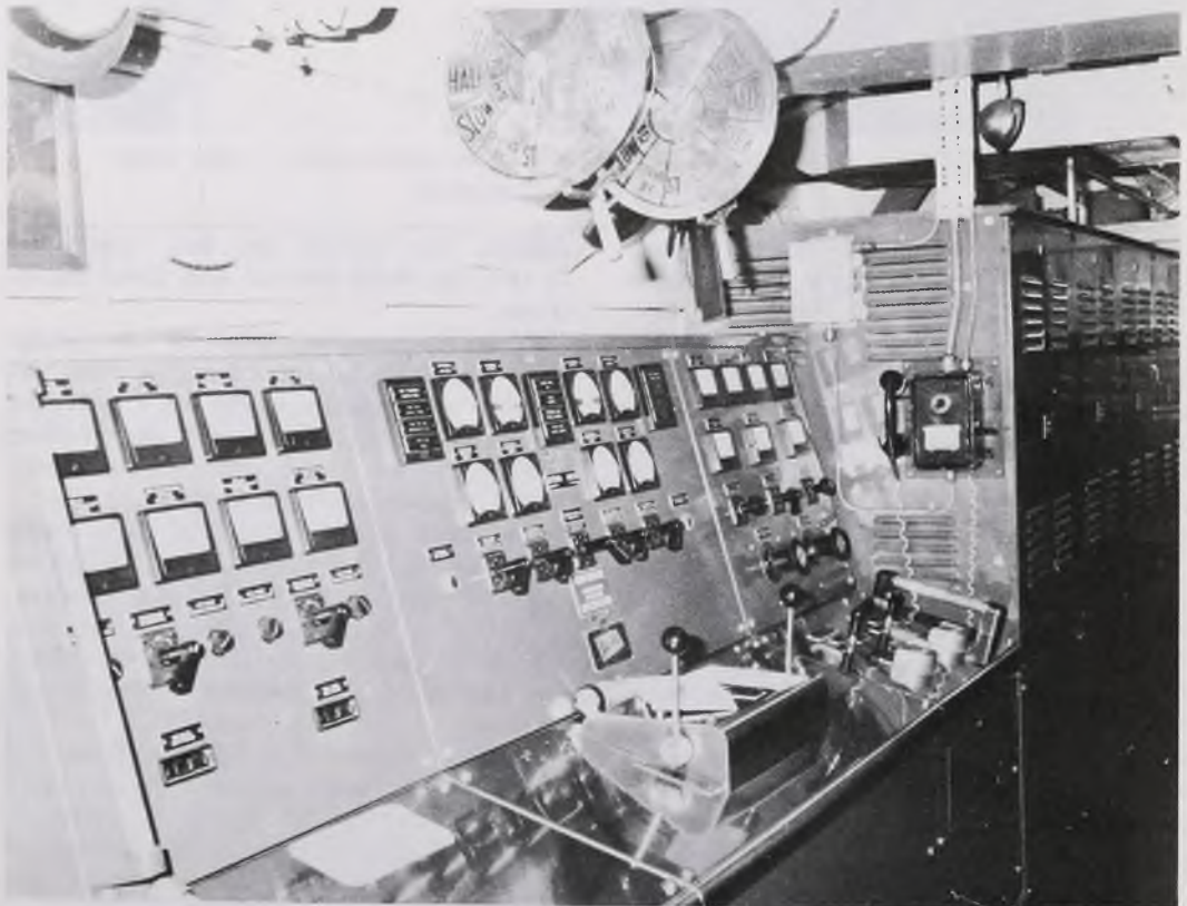
With full pilot house control, the engine room telegraphs read 'finished with engines', even though the diesels are roaring full speed ahead outside of the engine control station.
