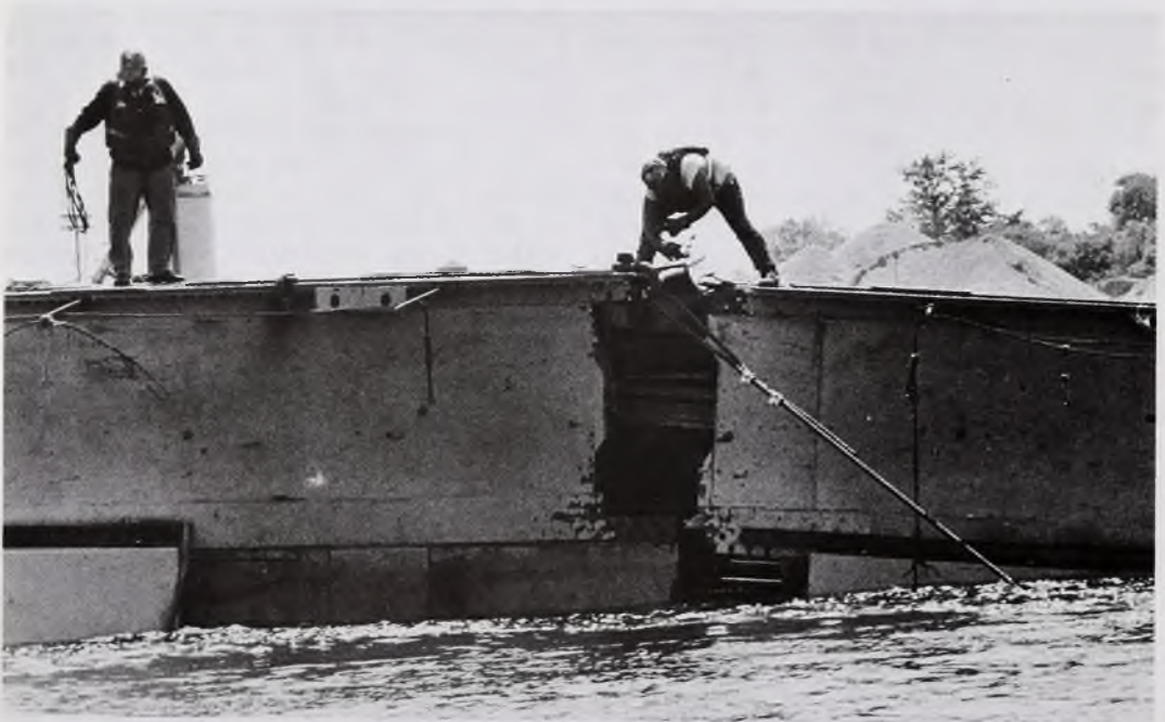
The SMITH rolled over in 40-feet of water and the bow section broke away completely and sank in deep water.
