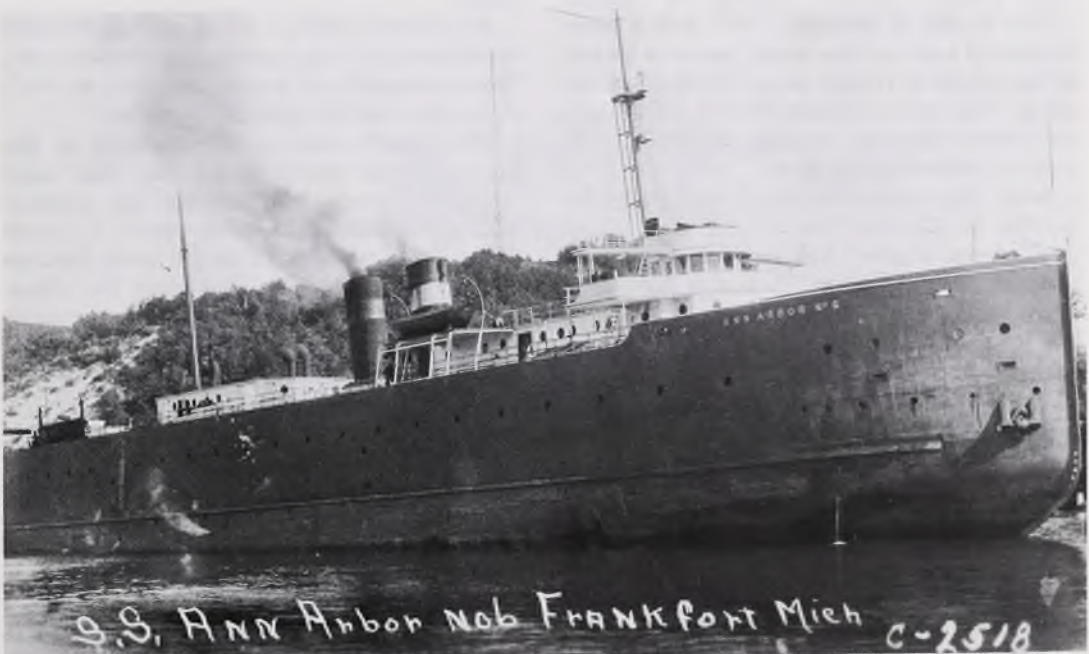
The ANN ARBOR NO. 6 could carry twenty six rail cars on her four decks.
