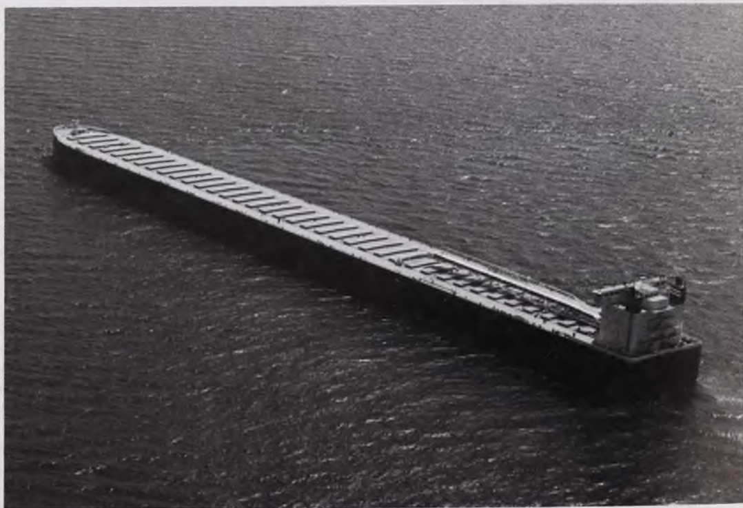
The INDIANA HARBOR'S maximum cargo capacity at 34' draft is 78,850 long tons of iron ore.
