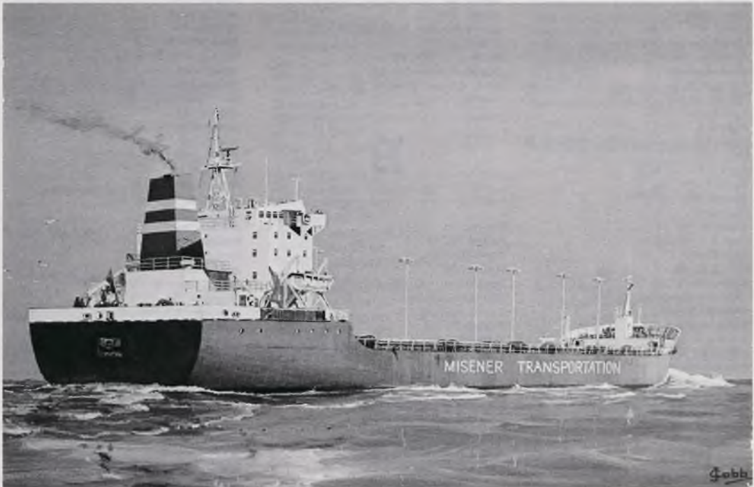
An artist's impression of the 33,000 tonne deadweight bulk carriers ordered from Govan Shipbuilders, Glasgow, part of British Shipbuilders, by Misener Transportation of Ontario, and Pioneer Shipping Ltd., of Manitoba. The vessels are of an advanced flexible design developed by Govan Shipbuilders, enabling them to be used either for Canadian Great Lakes operation or world-wide deep-sea trading.
