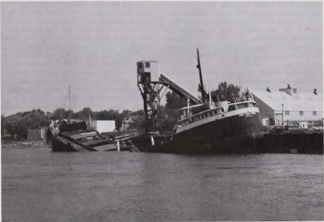
While loading salt, the NEW YORK NEWS (iii) buckled and settled to the bottom.
