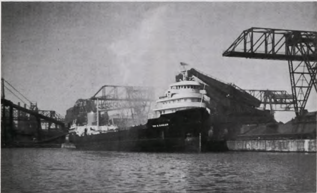
TOM GIRDLER at Republic Steel ore dock in 1967 after she was emptied by the only Hulett unloaders ever installed in South Chicago. Note the overhead coke conveyor at left, extending into Interlake's Federal Furnace.
