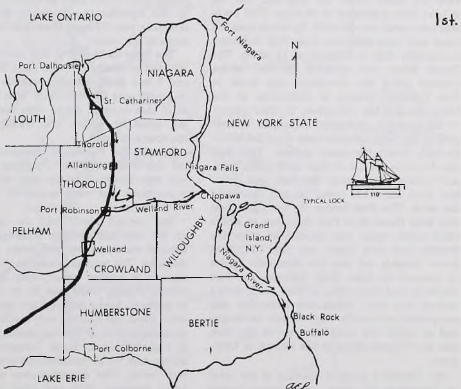
The first Welland Canal consisted of 40 locks, allowing vessels of 100 feet in length to use it.
