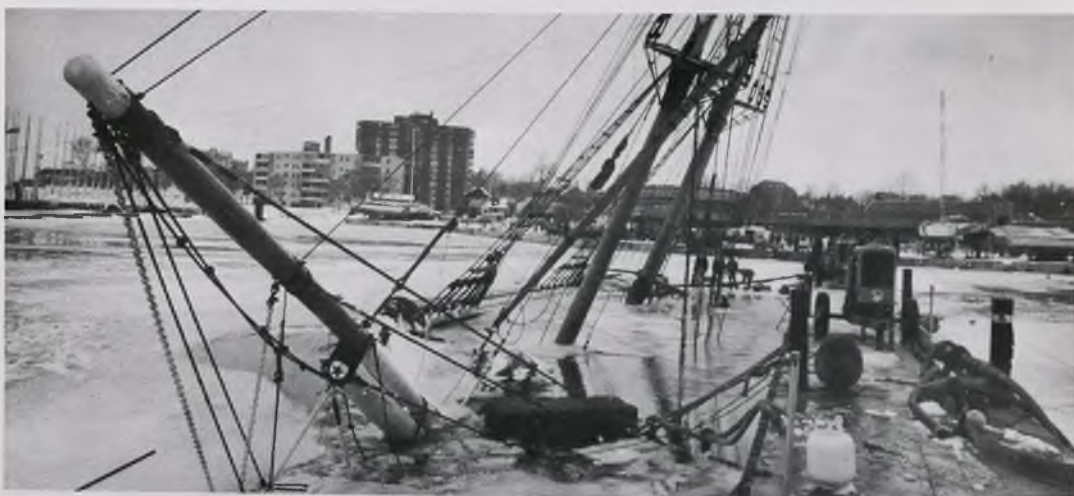
The bowsprit of the CIUDAD DE INCA rises above the waters of Portsmouth Olympic Harbor in Kingston, Ontario on January 10, 1986, as successful efforts to refloat the tall ship were carried out. Flotation bags and large pumps were used to raise the ship.
