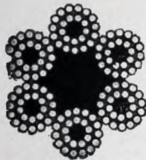
6 strands 24 wires for Mooring Lines
