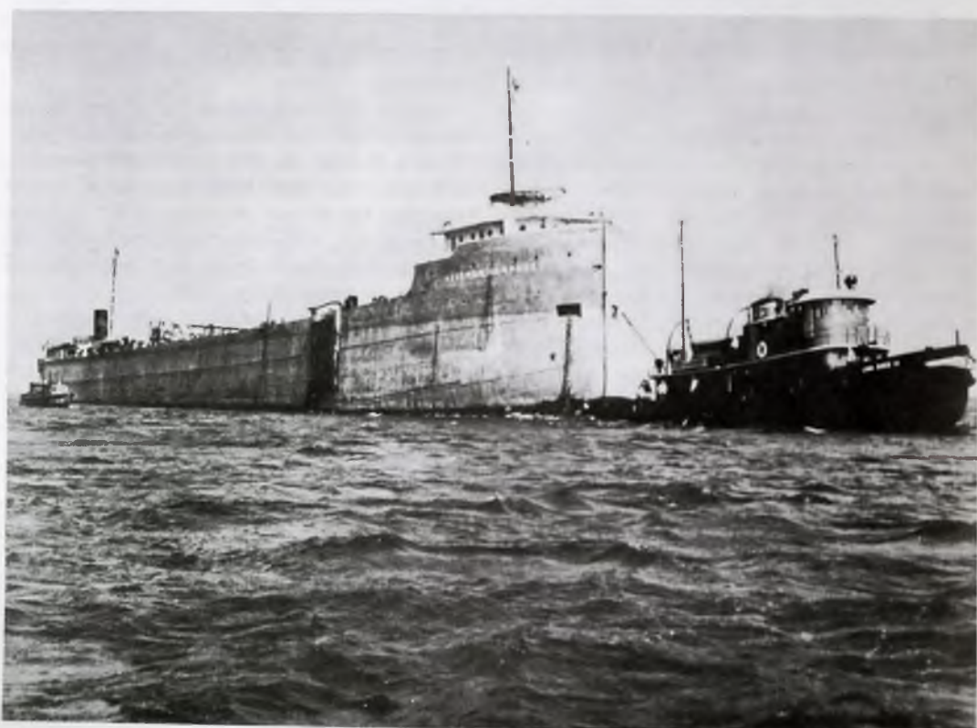
Top: The HUMPHREY was raised from the bottom in September, 1944. Bottom: Tug JOHN ROEN III towed the HUMPHREY to the shipyard for repairs after the "impossible" salvage was completed.
