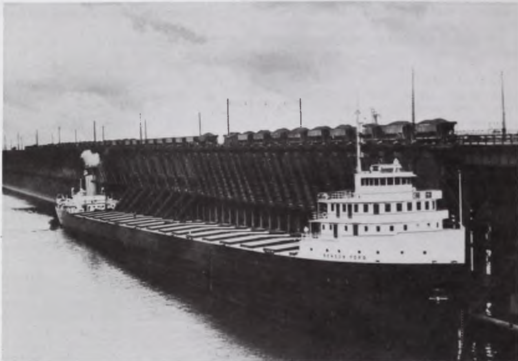
The BENSON FORD remained a straight-decker during her entire career. When built in 1924, she and the HENRY FORD II had a carrying capacity of 13,600 tons.
