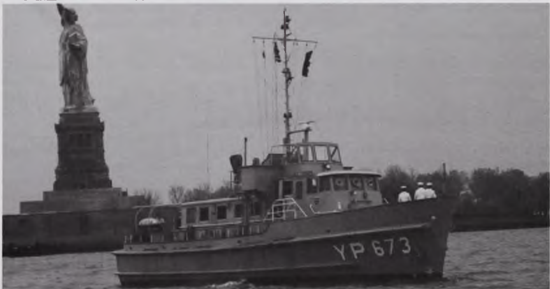
The PRIDE OF MICHIGAN in New York harbor on May 9, 1989. Built in 1977, the former yard patrol craft measures 80.6x17.8x5.3. She is powered by two Detroit diesels with a cruising speed of ten knots.
