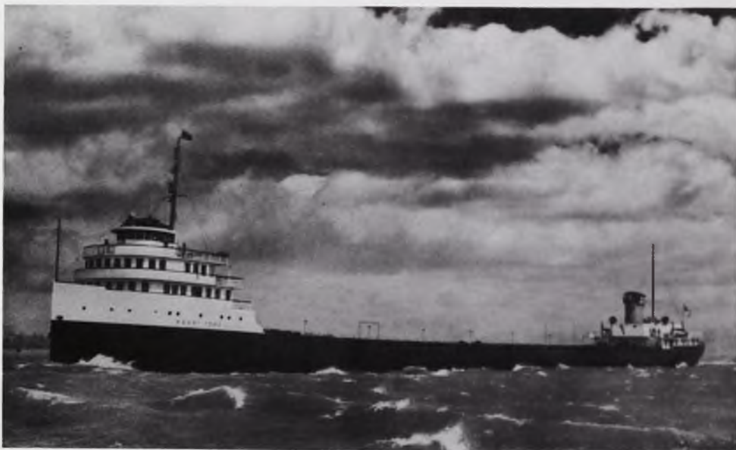
The HENRY FORD II was the first laker to be powered by a diesel engine and had completely automated electric winches, steering gear and heating.
