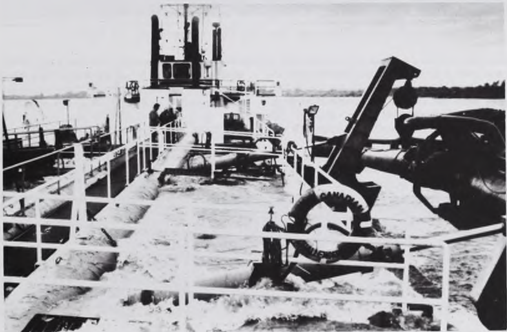
The HUTCHCLIFFE HALL was converted to a hopper dredge in 1971-2. The forward cargo hold was rebuilt as a pump room, leaving the other holds to serve as hoppers.
