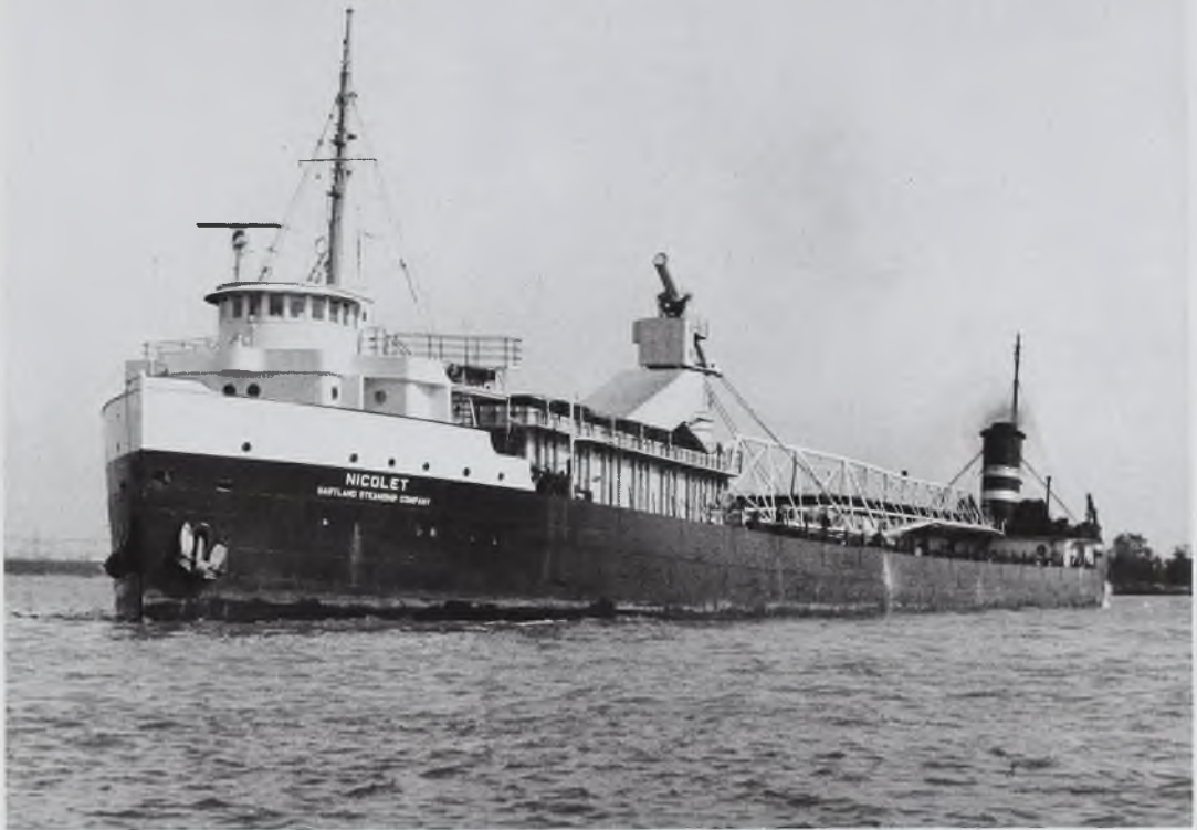
In 1965 she was renamed NICOLET and converted to a self-unloader.
