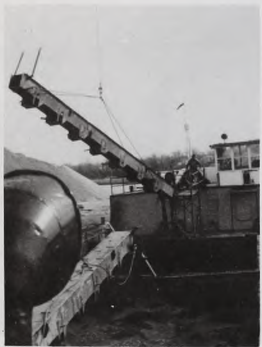
The screen is repositioned aboard the OSBORNE in preparation to pump another load of sand.
