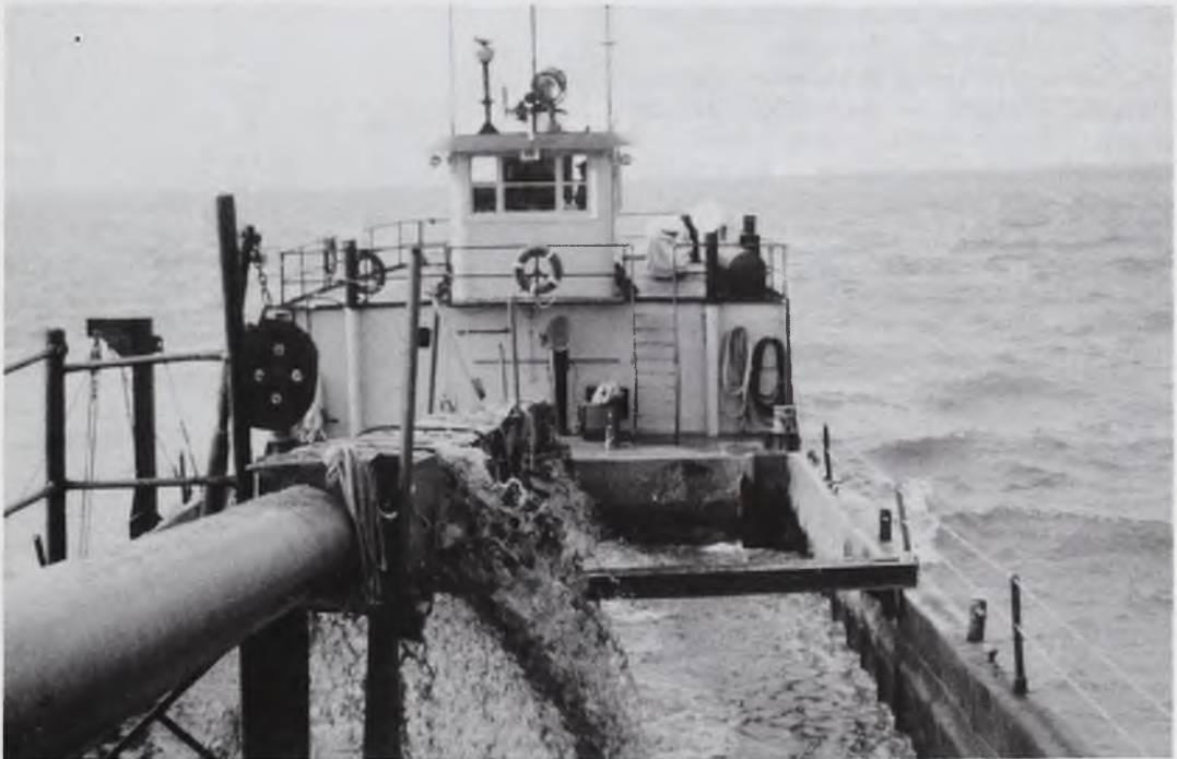
Top: A pipe with hood in lowered to the lake bottom to pump sand. Bottom: The pumped material flows through a screened trough along the vessel's centerline. Sand falls through screens into open-hatch cargo hold.
