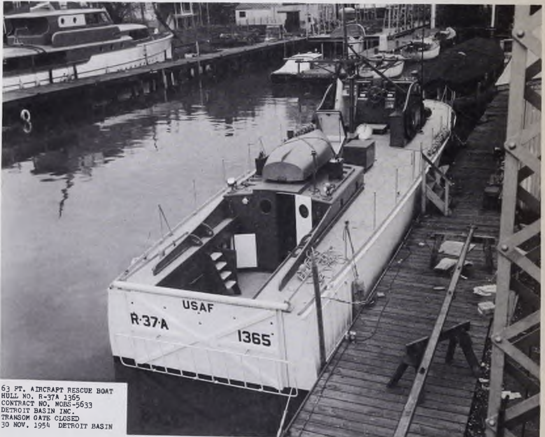
The 63-foot rescue boat finished with the transom gate closed.
