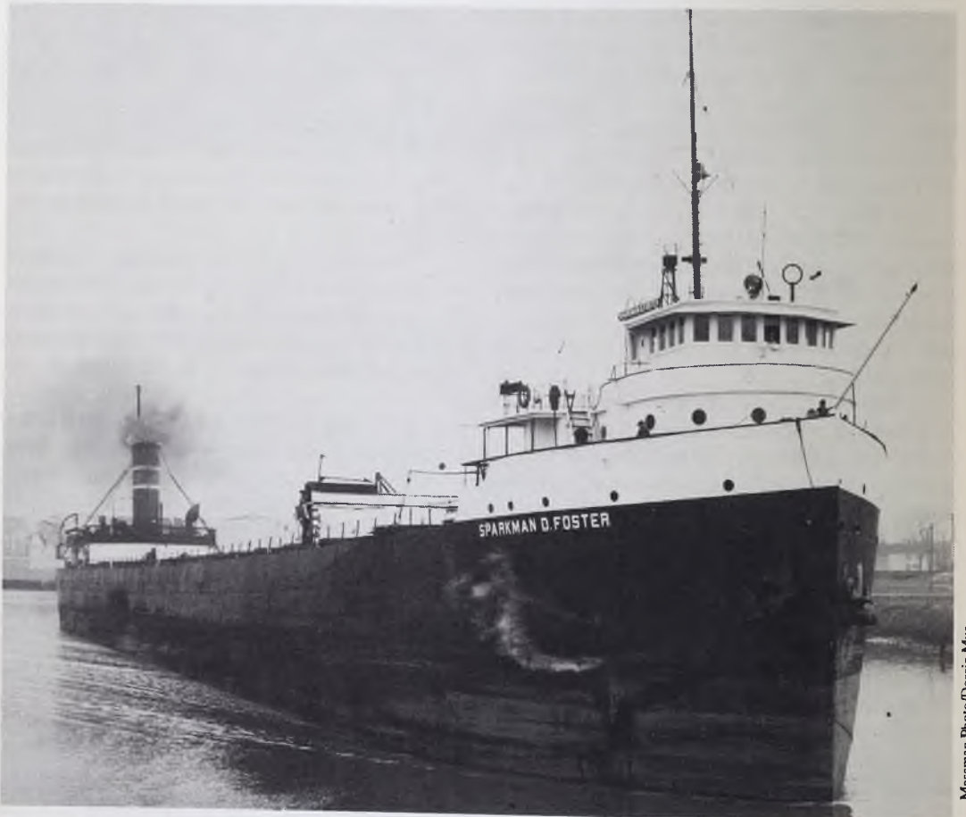
Top: The arrangement of the unloading rig on the COLONEL E.M. YOUNG was reversed so that the boom extended forward. Bottom: The YOUNG was renamed SPARKMAN D. FOSTER when she was sold to Browning family interests and reconverted to a straight-decker.
