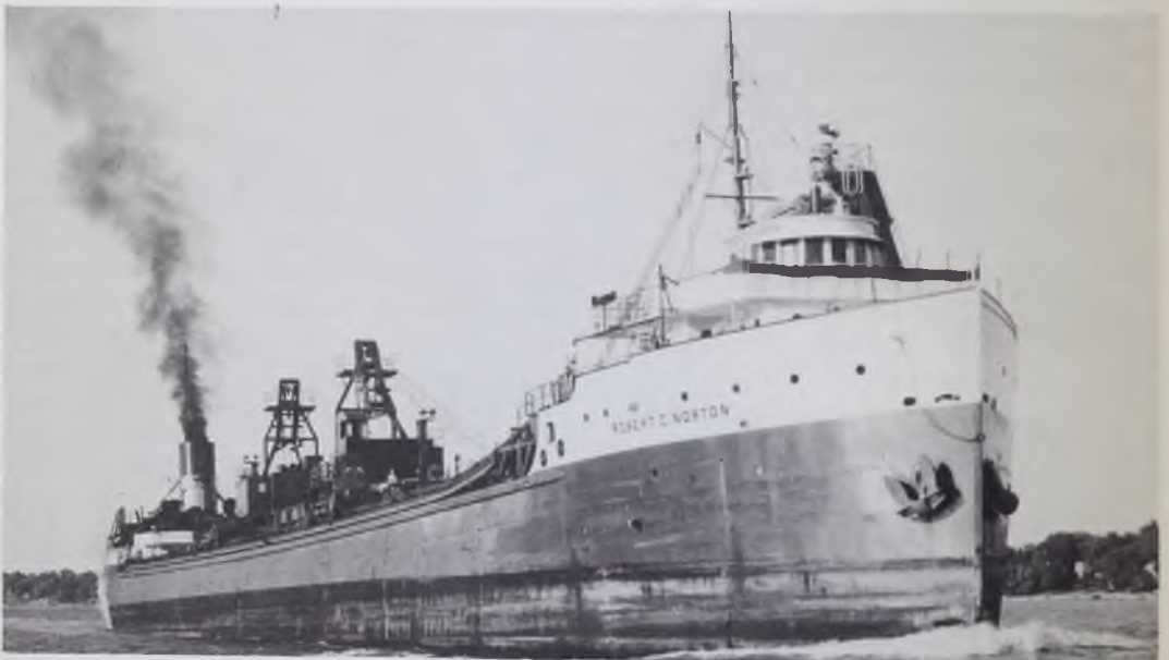
Two traveling cranes allowed the NORTON to place material farther onto the dock and did not materially reduce the cubic capacity of the vessel as would the installation of hoppers and conveyors in the hold.
