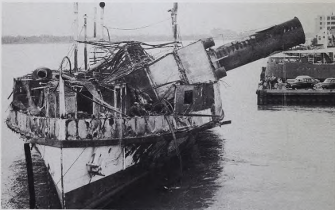
Top: Within minutes of igniting the oil-soaked wood decks, the PUT-IN-BAY was engulfed in flames. Bottom: On Sunday, October 4, 1953, the hull was towed back to Detroit to be cut up for scrap.
