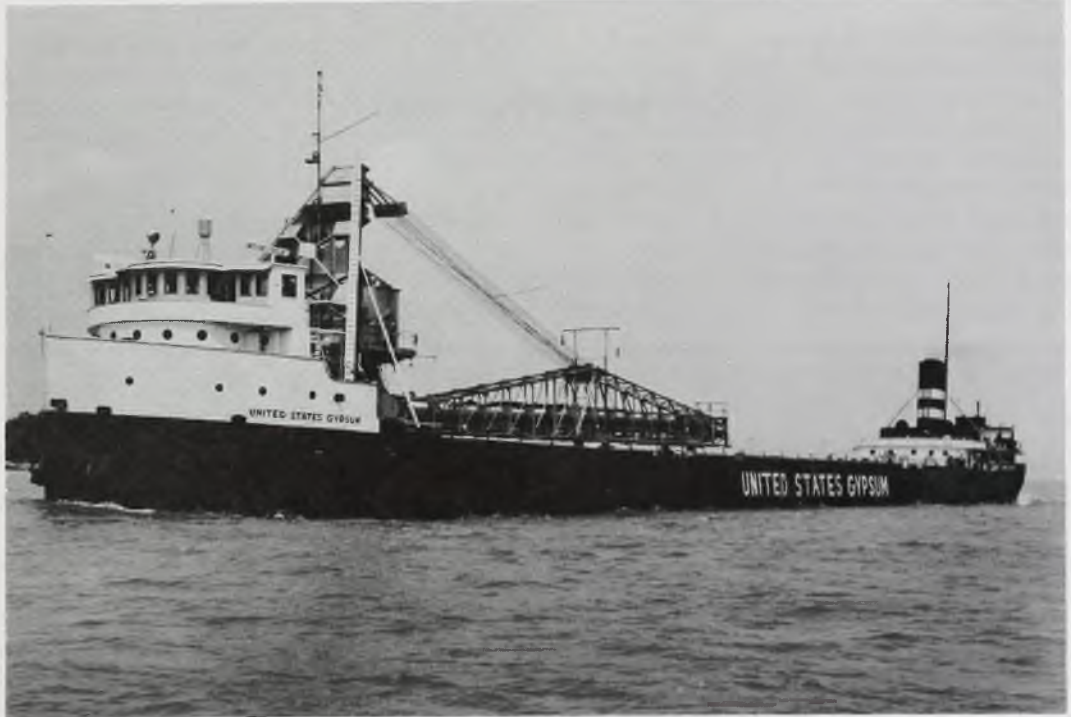
The UNITED STATES GYPSUM was built in 1910 and converted to a self-unloader in 1932.
