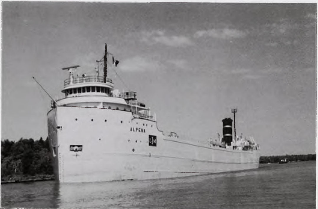
Top: The TREGURTHA carried 3,241,386 tons in a season. Bottom: The ALPENA was shortened 120 feet and converted to a self-unloading cement barge in 1990-1.
