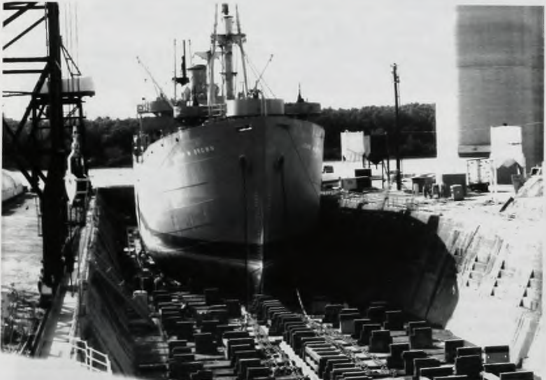
The JOHN W. BROWN at the Toledo (Ohio) shipyard drydock on June 12, 2000 undergoing her rivet replacement.
