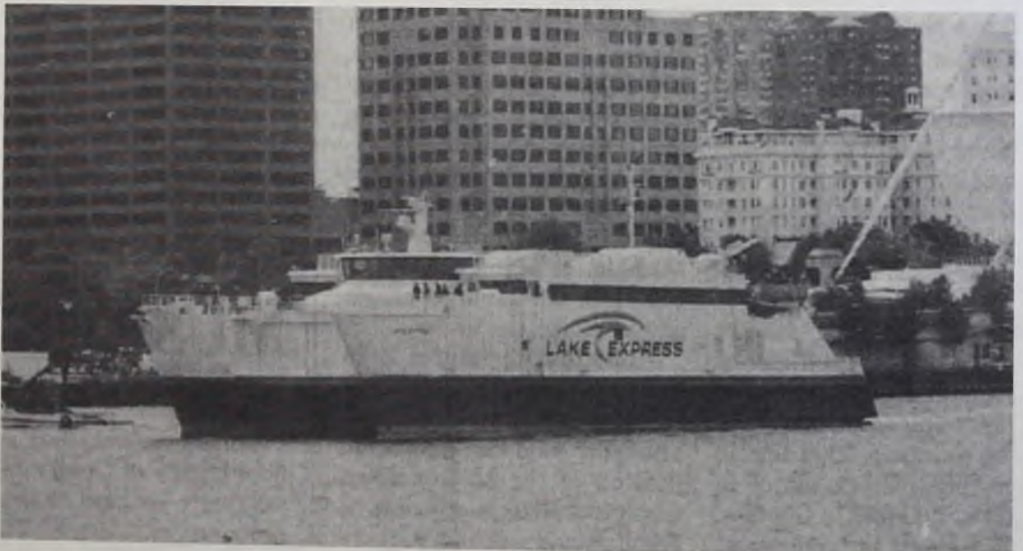
LAKE EXPRESS, the fastest commercial boat on Lake Michigan, began her runs from Milwaukee-to-Muskegon on June 2, 2004. She is a twin-hulled catamaran carrying a crew of 14, passenger capacity of 250 and vehicle capacity of 46. She is powered by four diesel engines generating 12,000 hp with a cruising range of 700 miles. She has a routine operating speed of 34 knots (40mph) and is scheduled to make 3 round trips per day from June to September and two per day from October to December. Photo by Ken Stevens. Associated Press. Reprinted from The Detroit News - May 30, 2004.
