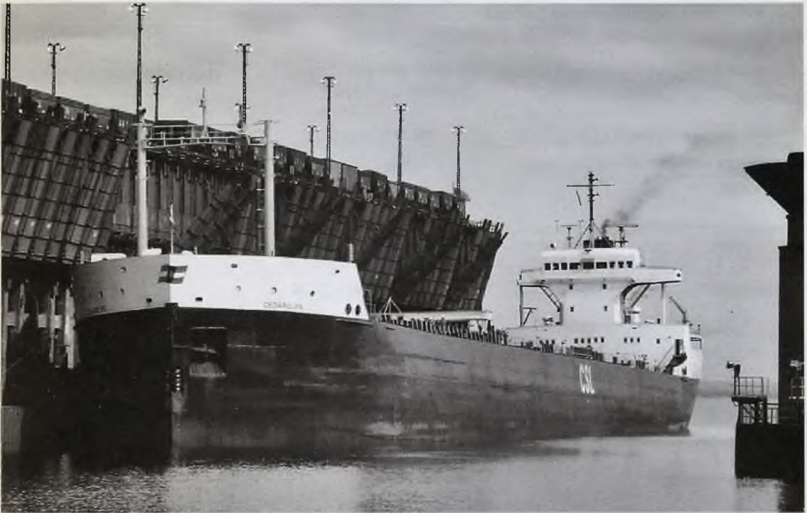
The starboard bridge wing of the CEDARGLEN was modified to fit under loading chutes.
