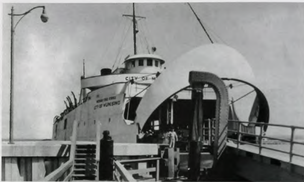
Bow Door is the CITY OF MUNISING, identical to the one fitted on the CITY OF PETOSKEY. Photo from the Dossin Great Lakes Museum collection.
