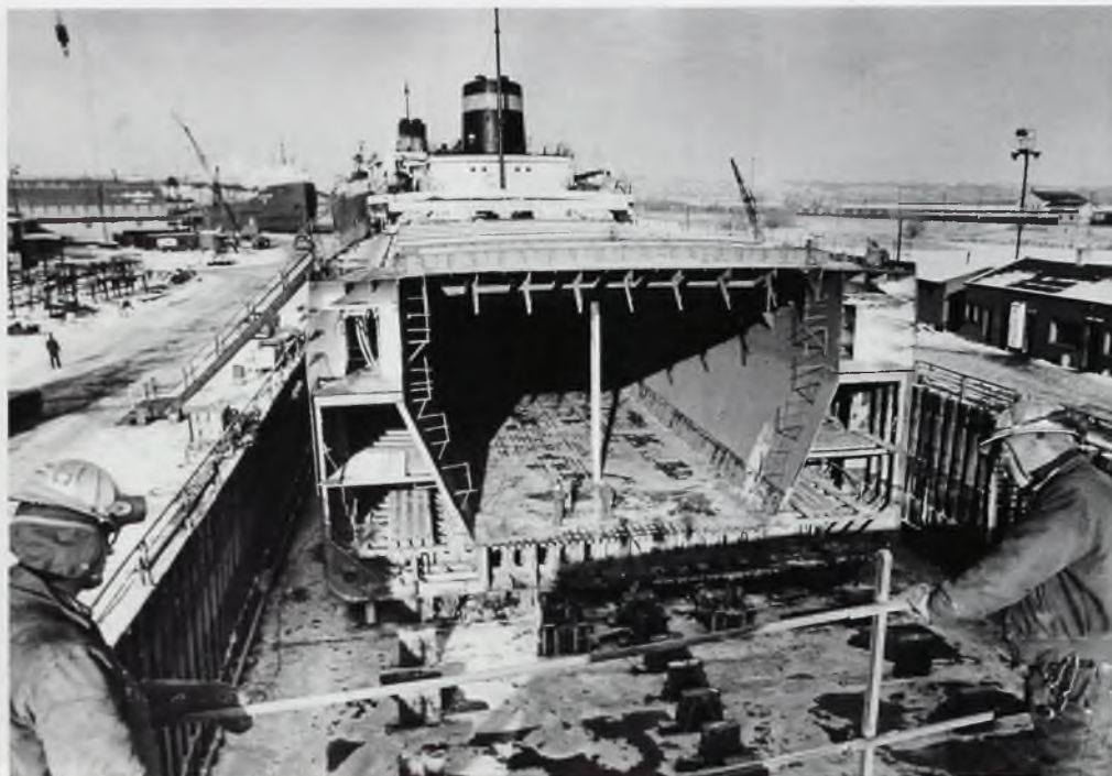
Lengthening of the CHARLES M. BEEGHLY at Fraser Shipyard.
